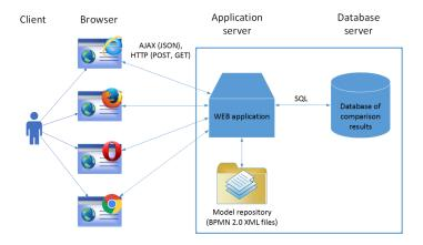
Fig. 1: Architecture of the BPMNDiffViz tool
