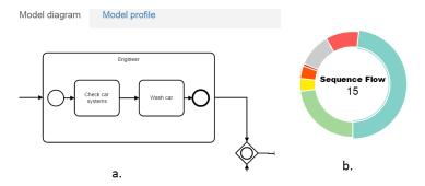
Fig. 3: Visualization of a BPMN model (this model contains 15 sequence flows)
