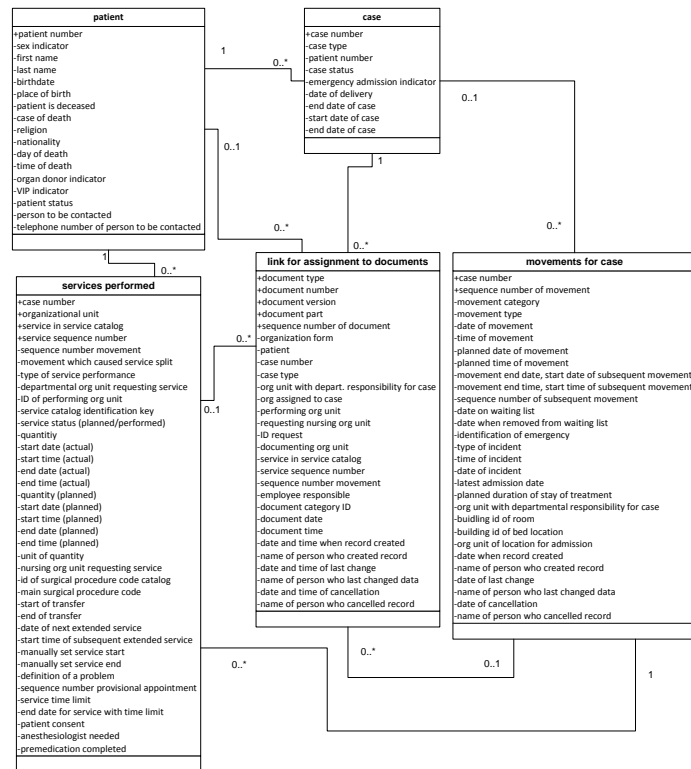
Figure 6: Linkage of medical documents to patients, cases, movements, and performed services. For each of them, multiple links may exist (link for assignment to documents class).
