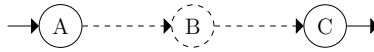
Fig. 5. Missing events: events “A”, “B”, and “C” have occurred in reality. Only events “A” and “B” are included in the log whereas event “B” is not included.
